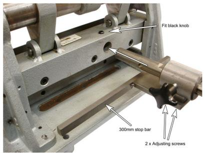
3. Fit the length stop bar to rear of machine by inserting the stop bar assembly into the 25mm diameter hole in top blade support block. Push the stop (300mm bar) against the top blade. (This bar can be adjusted by undoing the two screws underneath). Align the edge of the knurled circular block with the zero on the scale which is attached to the 25mm diameter bar and tighten the black knob on to the assembly.
