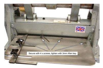
5. Place guide plate on front of guillotine and do up the 4 screws with 3mm Allen key.
