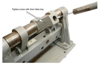
4. Insert the pull down bar into the hole as shown above and do up the screw with 3mm Allen key.
